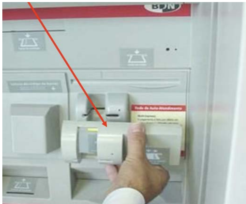
Another example of a skimming device being placed onto the card reader.
